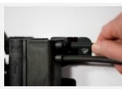
3. Disconnect electrical connectors from the unit harnesses
