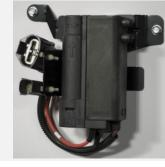
2. Disconnect washer hoses from inlet and outlet of the unit
