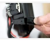
Remove electrical connectors from the bracket by lifting white locking tab while pulling connector outward.
